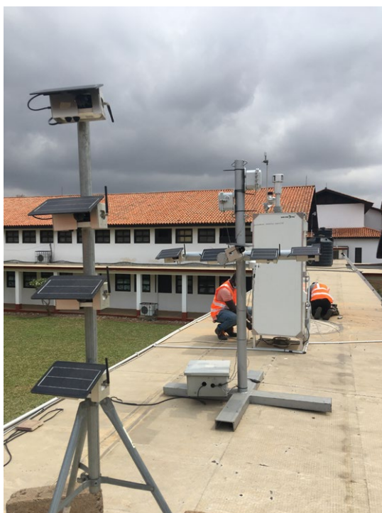
FIG. 4.4A Collocation at UG of LCS (located in the two posts in front of the picture) with fixed reference-grade monitors, which are located inside the white shelter at the back of the picture (Jessica Pourraz)
