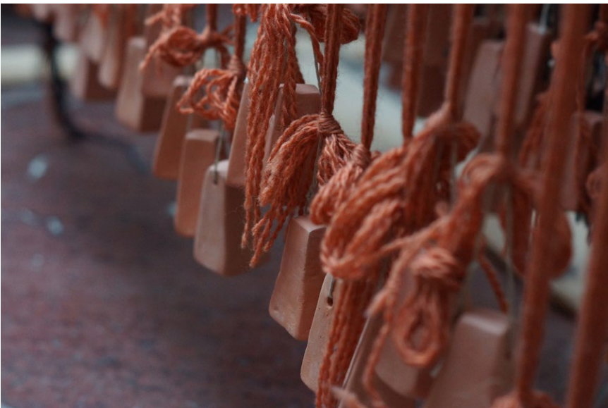
FIG. 1.2 Clay weights attached to the warp on the warp-weighted loom (photo by Viktoria Lubomski in 2019)
