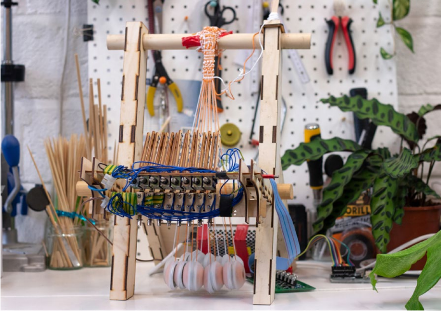
FIG. 12.1 The Live Loom, a hybrid, open hardware, warp-weighted hand loom, with 16 computer-controllable warp threads (photo by James Hendy)
